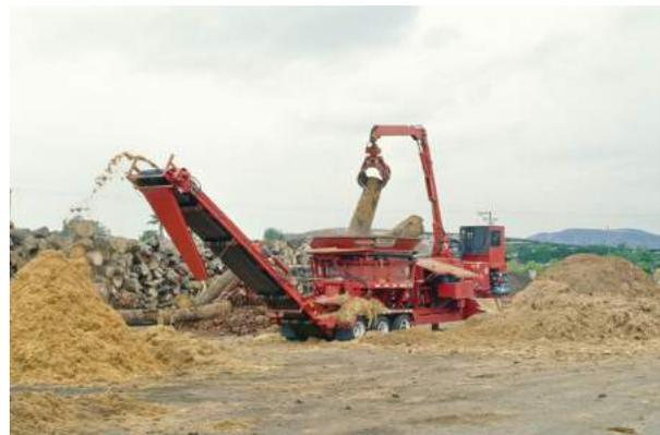
Figure 26. At the approved disposal processing site, grind up all palm material into pieces no larger than 1 1/4 inch square (D. R. Hodel).
